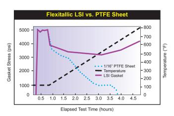
The "LSI" gasket retains more of its initial stress or tightness, even when subjected to high temperatures, unlike PTFE sheet gaskets.
