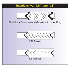
Extruded filler allows "LSI" to be used with lightly loaded flanges. "LS" style is also available.
